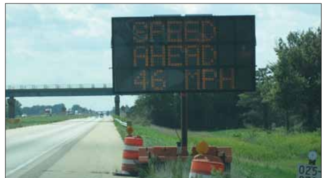
Figure 1. A portable changeable message sign providing downstream traffic speeds from sensor data.
